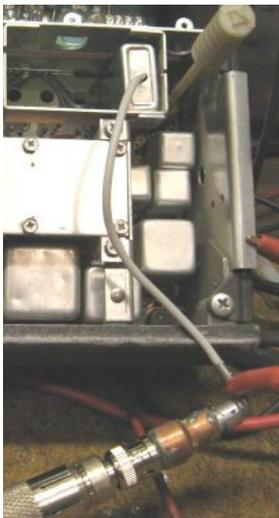
does not have a direct path to chassis ground you need to do that. A jumper clip from the coax shield, to the ground should do the trick.
