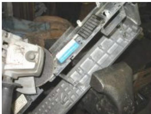
The correct type cage (robbed from an old high-band chassis) was replaced with small bolts and nuts.
