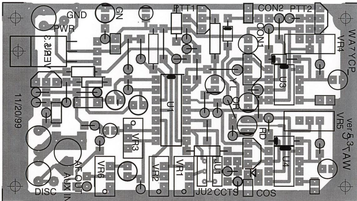
Notes: The silkscreen (below) shows the tail and time-out (LED) indicators as orange and red, respectively. Since red is a PTT/tail function, the two colors are now swapped on the boards. The board
