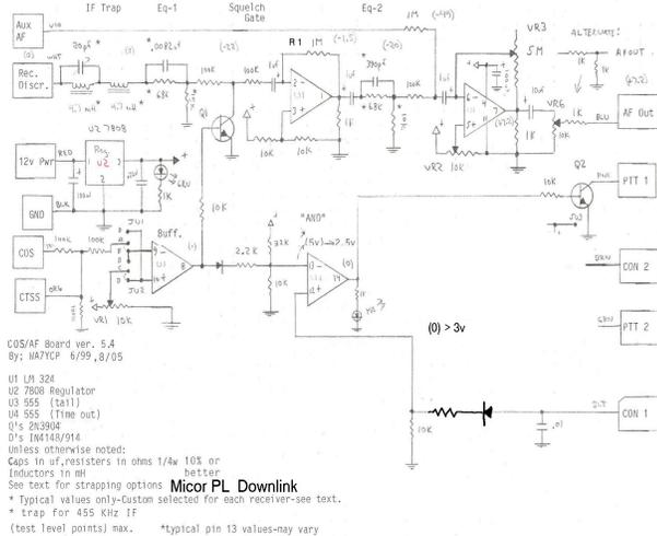
For the Spectra-Tac version the downlink configuration is show here. If you do not need the time out time it can be left on the board (intact) but disabling it by adding a jumper (solder bridge) at the green points. See the (separate) drawings for more details.
