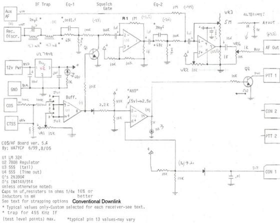
If you wish a **conventional** interface to use with any PL deck (decoder) connect it to CTCSS input. This way also supports micor H.U.B. (closed loop) control. This will make both PTT and audio paths protected.
