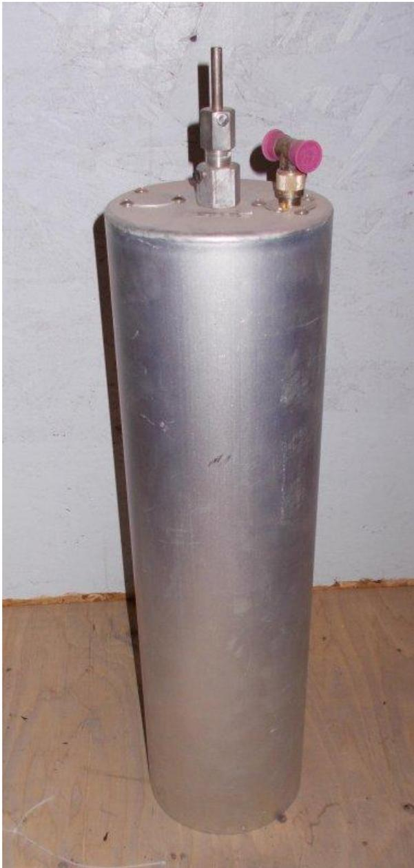
Cavities come in various physical sizes but can be made electrically for the same band. Also, they are made in the different RF bands for both commercial and amateur use. In many cases used commercial band cavities can be tuned for the amateur band. It depends on the cavity design, specifications and "Q" of these devices.
