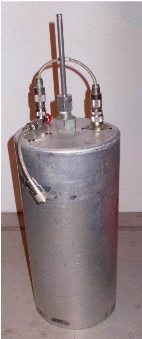
Shown here is the final "product" modified for the amateur band. Shown here in the "high" mode, AKA high pass mode with the 1/4 wavelength of coax "T" connected to the cavity's RF port (connector). For the low pass mode one just leaves this T extension out.
