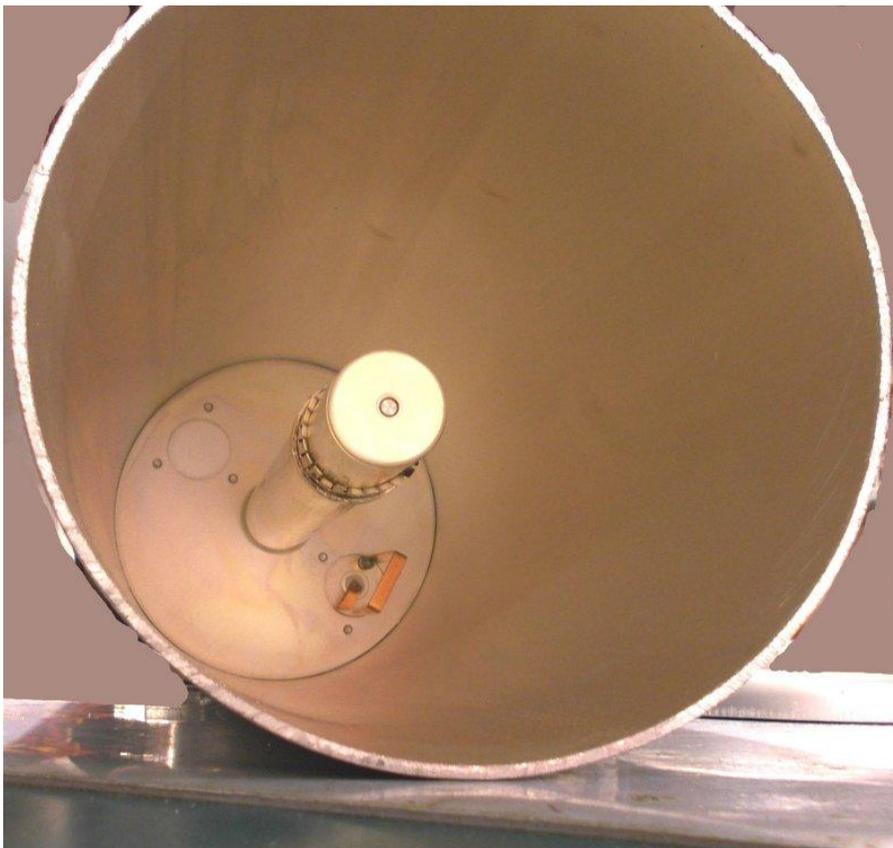
Shown here is a close-up of the stub, piston and coupling loop after the cutting is done.
