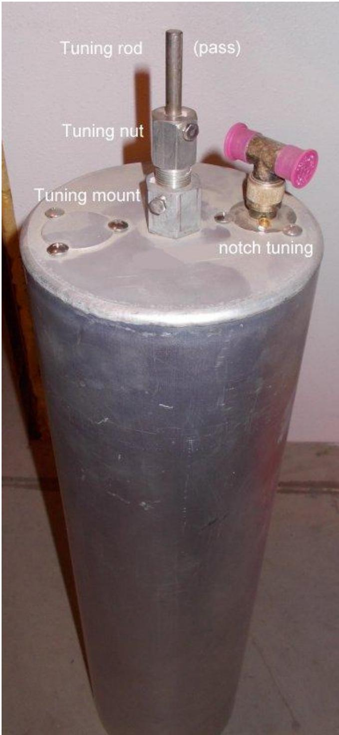
This type of cavity is a “BpBr”, meaning, band pass / band reject.
