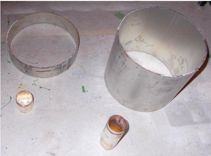
Shown here is the leftover cavity and stub materials. As you can see the Author performed 2 cuts to be sure the correct frequency spread was obtained. In addition, the Author assembled the cavity enough to verify correct tuning range was realized. The reason is you don't want to over-cut and make the parts too short and useless.
