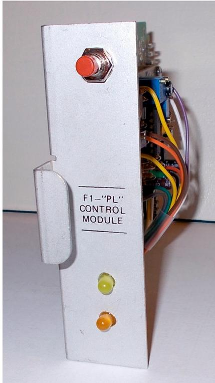
Here's the finished cor board, installed on the card, aligned, tested and ready for deployment (in service) in the Spectra-tac receiver unit. For maintenance tracking each card is serialized. This particular card needed the monitor button added. Also, the timer and AF settings are indicated to be set.
