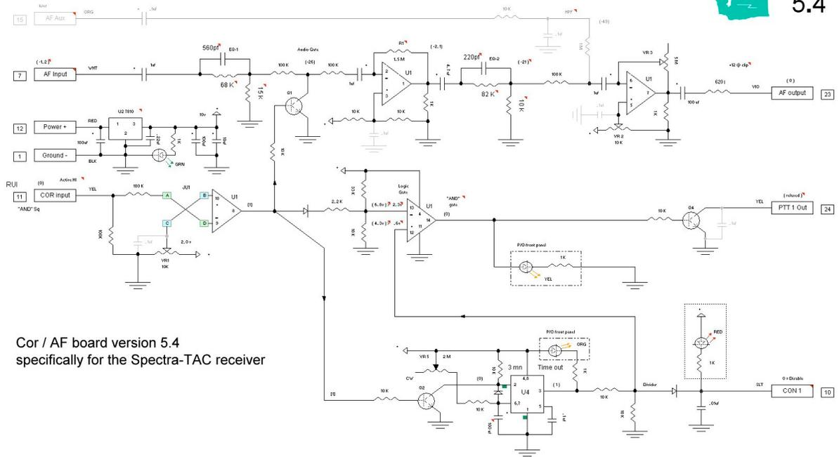
Cor / AF board version 5.4 specifically for the Spectra-TAC receiver
