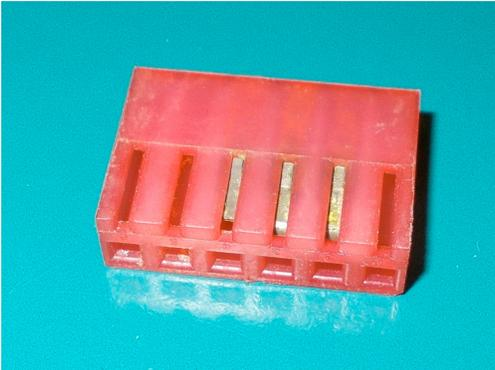
A problem found was intermittent power out. It was trouble shot to a badly corroded plug (and jack) on the interconnect board. P1004. Only three points are used, the A+, A- and control voltage.
