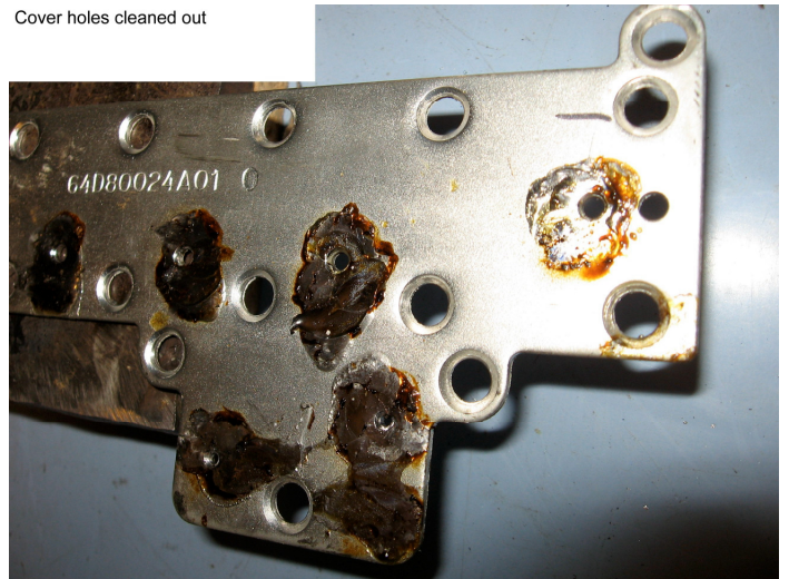
Cover holes cleaned out
