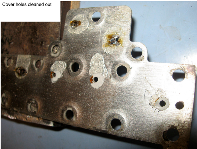
Cover holes cleaned out
