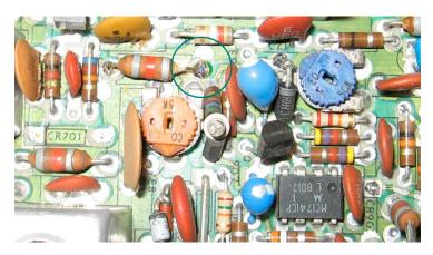
In some cases the leads may be not straight, plus one may be too short to come back into the eylet of the PCB. If its close you can flood the eyelet so it flows through the hole plus, add a little solder on the component side as shown here, with the teal circled area.
