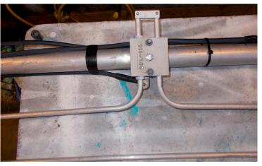
Here's the broken element on the left. A normal element is on the right.
