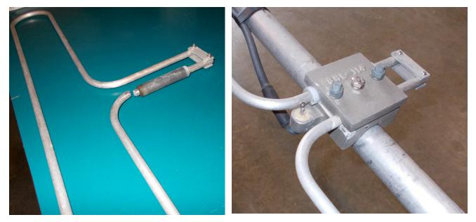
Taking the element off the array shows the back plate. Below are some close-ups on the center coax connection point for each element.
